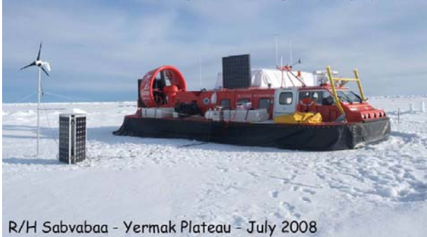
Wind Generator and Solar Panels are powering an autonomous drifting seismic profiling buoy - under test
